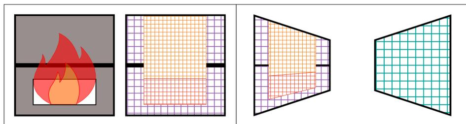
Figure 2: Illustrating the discretisation of an emitter into protected, unprotected and external elements and a neighbouring building's elevation into receiver elements.
