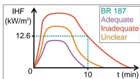
Figure 3: Illustrating the need for a comparative method for IHF curves
